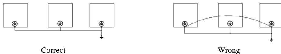
Figure 3-8 Grounding Wire Connection Sketch Map
