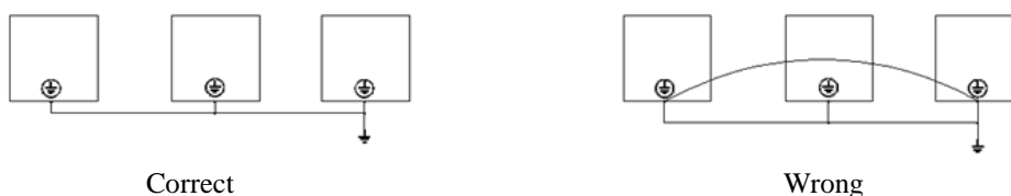
Figure 3-8 Grounding Wire Connection Sketch Map
